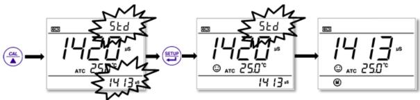
If return from calibration mode without calibration, press key to return to the measurement mode without calibration.
