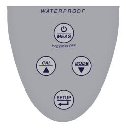
**Note**: In the calibration mode or the parameter set-up mode, press for return to the measurement mode, then press to turn off the meter.
